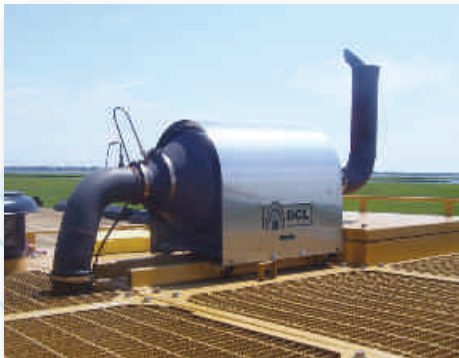
A MINE-X SOOTFILTER® DPF installed on a Caterpillar 245D Excavator
