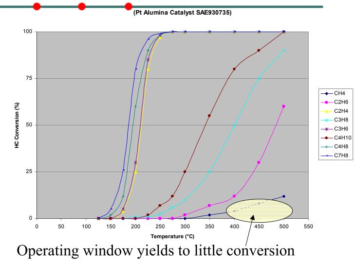
Need to install catalyst upstream of turbo Need to use another type of catalyst
