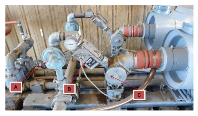
Figure 3: Regulators (A), solenoid operated gas control valves (B) and Impco Carburetors (C)
