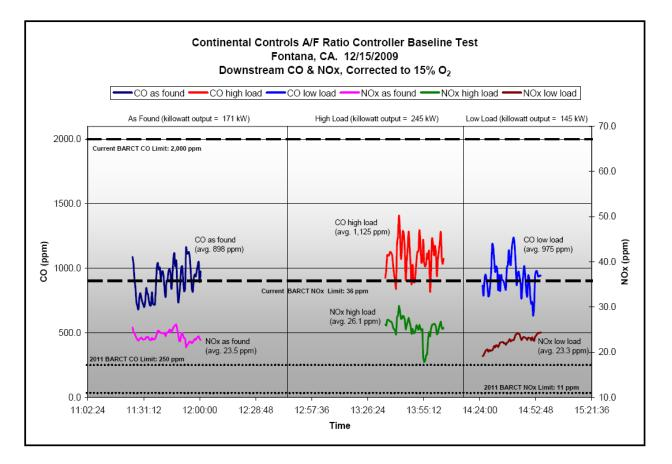
Figure 8 (above) and 9 (below): Baseline Emissions Data. Note fluctuations in the "steady-state data"
