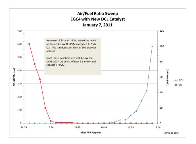
Figure 21: Sweep of Air/Fuel Ratio Setpoint from January 7, 2011 after apparent breaking-in or "de-greening" of the catalyst.
