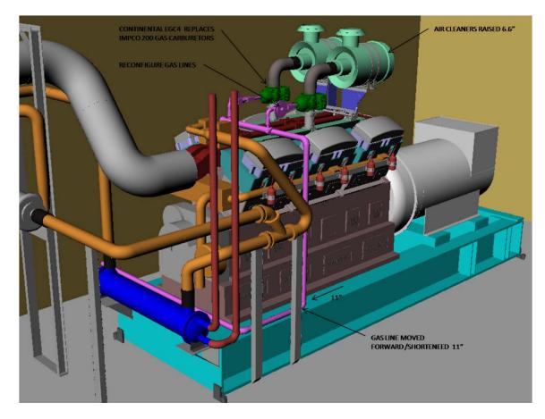
Figure 10 (above) and 11 (below): Preliminary Installation Drawings
