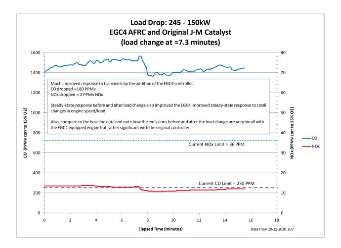
Figure 17: New EGC4 Controller and Old Catalyst showing reduced upset to emissions from a load change and steadier performance overall
