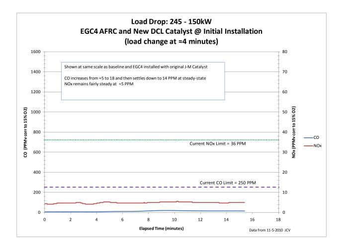
Figure 18: New EGC4 Controller and New DCL Catalyst showing initial performance
